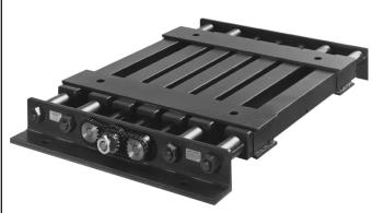
The DD-100 Series is for use with motors having a fixed diameter pulley. This series should be specified where heavy shock loads or vibration is generated, such as Rock Crushers, Vibrating Feeders or Screens, Foundry Shake-outs and similar equipment. Motors as large as 500 HP have been successfully mounted on these bases.
